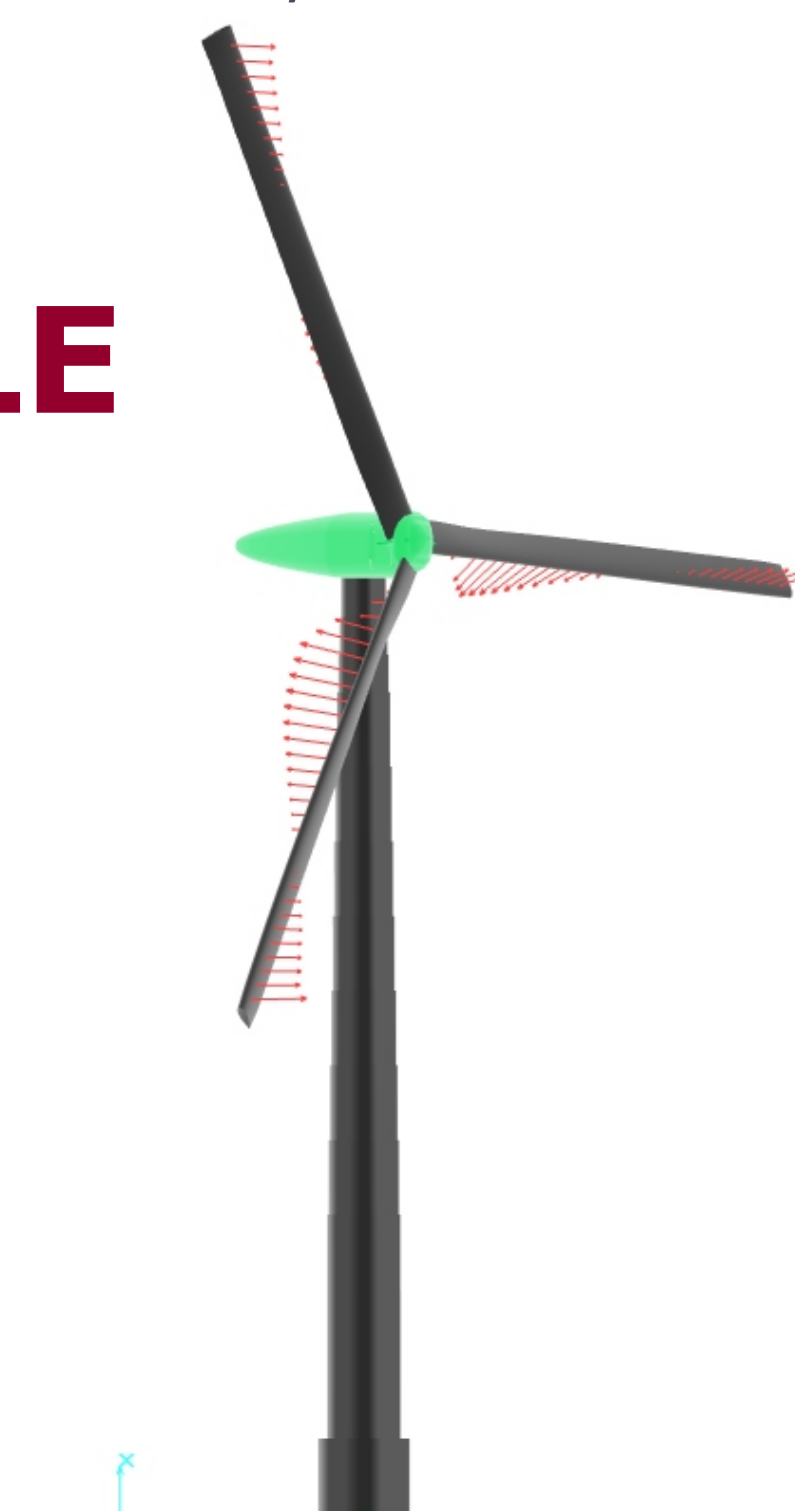
Wind turbine multibody model, with visualization of aerodynamic loads on the blades
