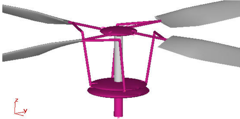
Figure 2: DYMORE model of the SASIP hub setup.
