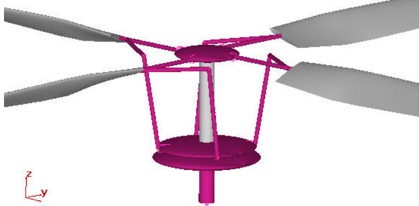
Figure 2: DYMORE model of the SASIP hub setup.
